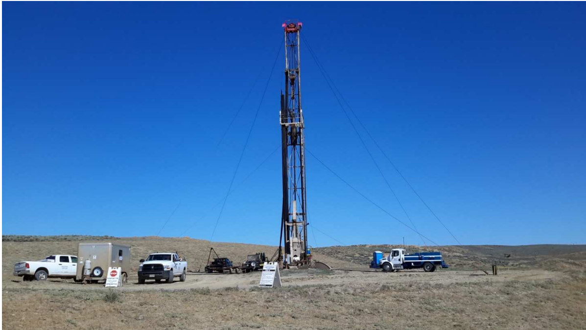
A Silvertip well being worked-over, wellbore being cleaned out and hydro testing the tubing
