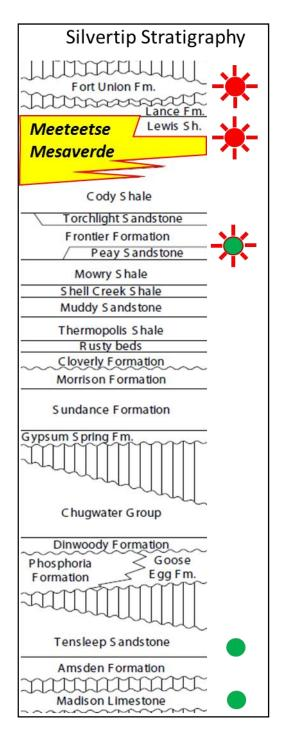
Two well recompletions were carried out in wells that had originally targeted the Frontier formation with perforations into the shallower Mesaverde and Meeteetse formations to extract behind pipe gas.
