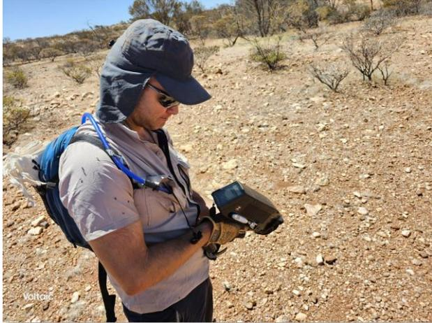
Laser induced breakdown spectroscopy (LIBS) handheld analyser for direct Lithium detection
