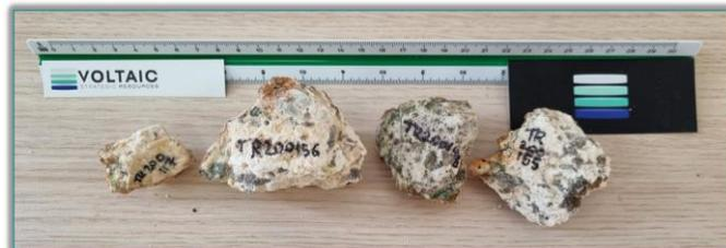
Rockchip samples (80) will undergo multielement analysis and appraisal of fractionation to assist with LCT vectoring.
