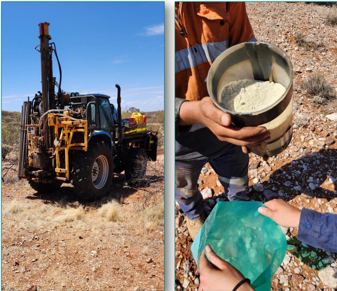
Figure 2: Auger vacuum drill rig at Paddys Well
