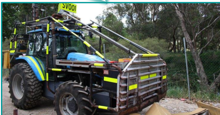
Typical auger vacuum drill rig. Source: Strataprobe Pty Ltd
