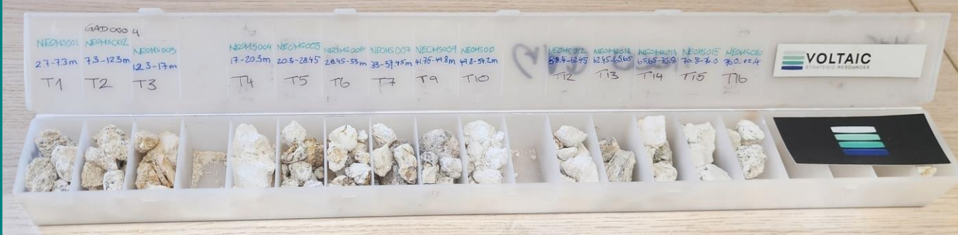
Historical core samples with anomalous REEs within clays
