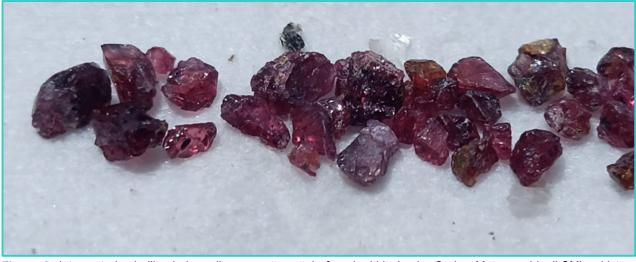
Figure 8. Interpreted rubellite / almandine garnet crystals found within Leake Spring Metamorphic (LSM) schist and rubellite/pegmatite contact (Akira prospect, ANDRC056, metre 43) <sup>3</sup>
