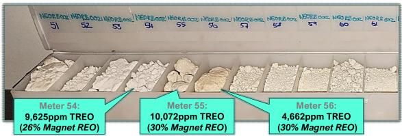
Figure 12. Chip tray photo of NEORB002 significant intercepts.
