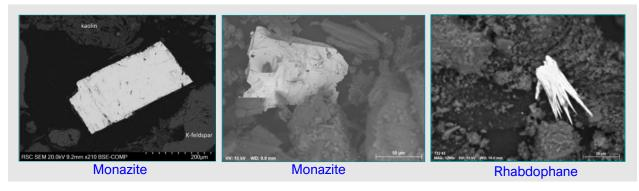
Figure 13. Monazite & rhabdophane (REE phosphate) crystals identified from SEM analysis of REE-enriched clay samples from historical drillhole GAD0004
