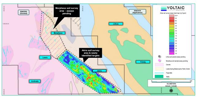
Figure 9. Akira prospect regional soil sampling survey – lithium in soil anomaly
