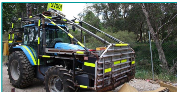
Figure 5: Typical auger vacuum drill rig. Source: Strataprobe Pty Ltd
