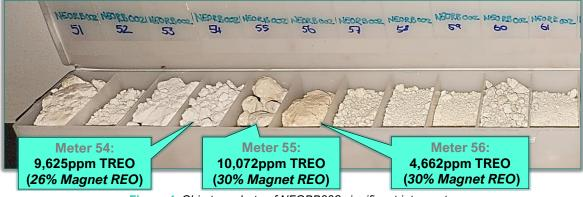
Figure 1. Chip tray photo of NEORB002 significant intercepts.
