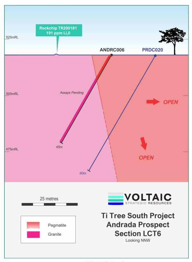
Figure 8. ANDRC006 (LCT06) Cross Section
